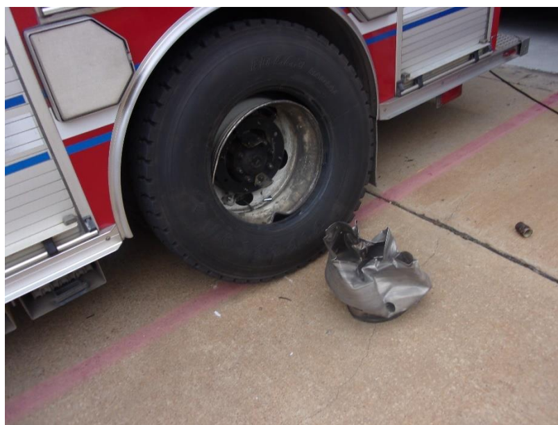
Photo 1: Apparatus tire that came off the wheel rim while being refilled with air. (Courtesy of the fire department)
