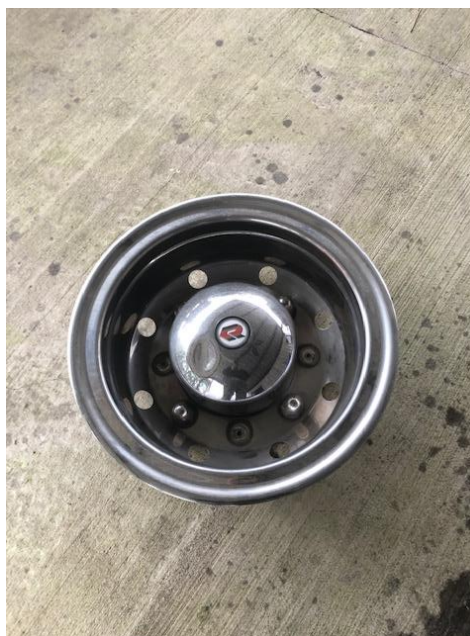
Photos 3 and 4. Apparatus tire that came off showing rim deformation and simulator/hubcap from passenger side of Engine 4.
