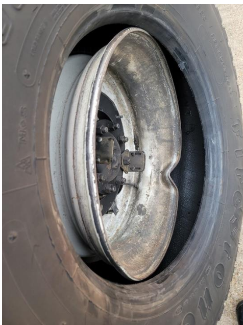
Photos 3 and 4. Apparatus tire that came off showing rim deformation and simulator/hubcap from passenger side of Engine 4.
