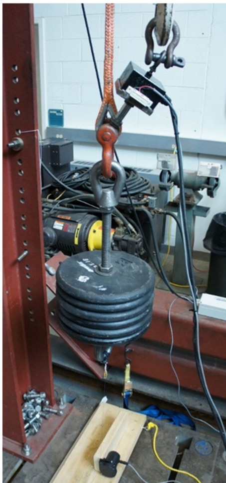
Fig. 2. Nystron rope "break-in" configuration.
