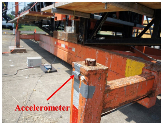
Fig. 4. Accelerometer on the outrigger pad column.
