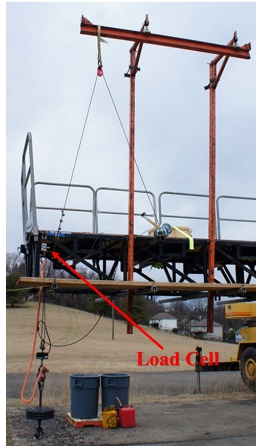
Fig. 3. Dead-weight drop test configuration.
