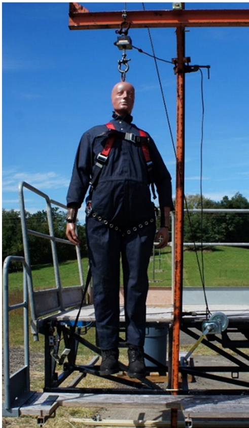
Fig. 5. Fall-arrest scenario configuration.
