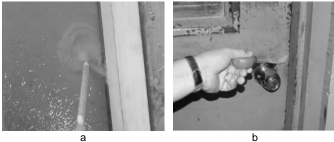
Figure 3. (a) Picture of the emissions from a smoke tube lingering inside the room because there is no positive pressure (system off). (b) Picture of smoke leaving the room since positive pressure is causing contaminant to be pushed out of room (system on).
