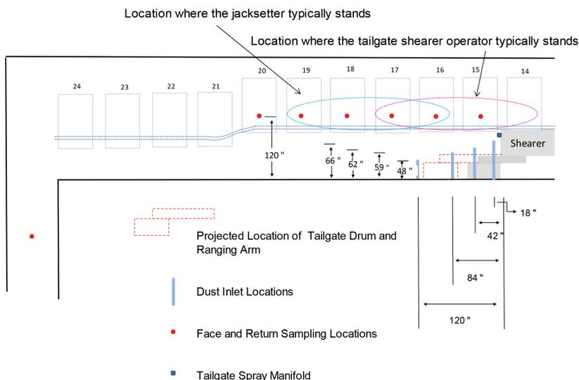
**Figure 1** – Diagram of sampling positions for dust inlet locations for tailgate manifold testing in longwall test facility.
