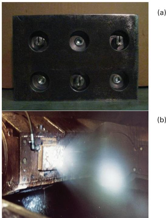
**Figure 5** — (a) NIOSH fabricated spray manifold. (b) The spray manifold mounted on the tailgate side of the shearer.
