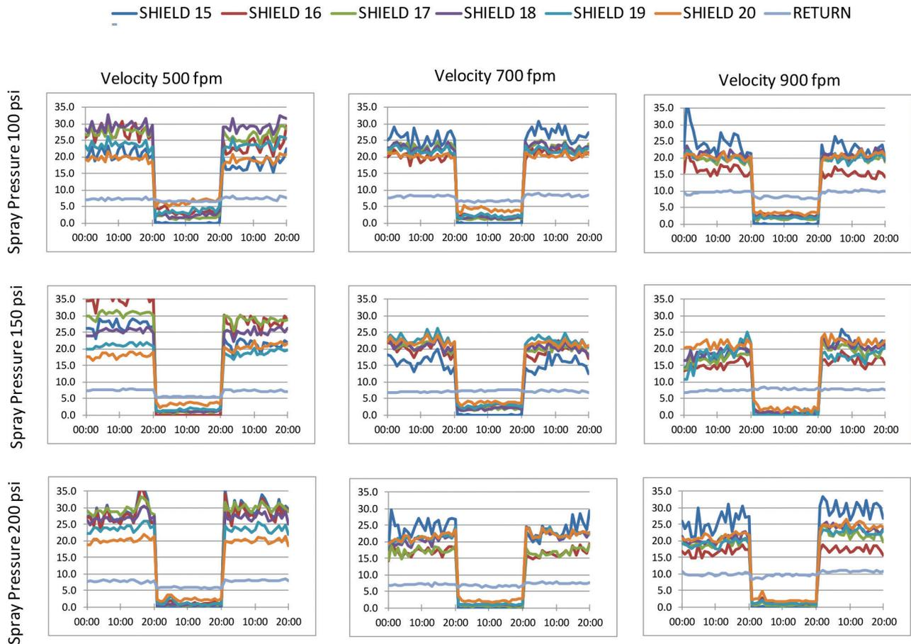
**Figure 4** – Instantaneous dust concentrations in  $\text{mg}/\text{m}^3$  for tests conducted with 40-20 spray nozzles.
