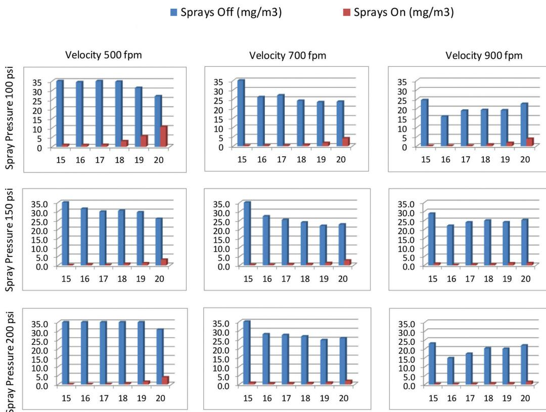
**Figure 3** – Dust concentrations in  $\text{mg}/\text{m}^3$  with spray nozzles off versus activated for tests conducted with two tailgate manifolds and four SS 65-15 flat fan sprays.
