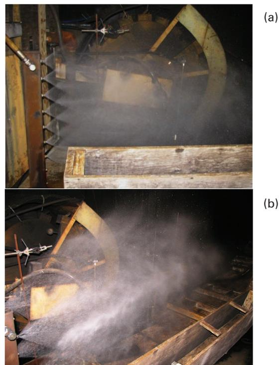
**Figure 2** – (a) Spray plume from the SS 65-15 spray manifold system and (b) BD3 spray manifold system attached to the tailgate end of the shearer.
