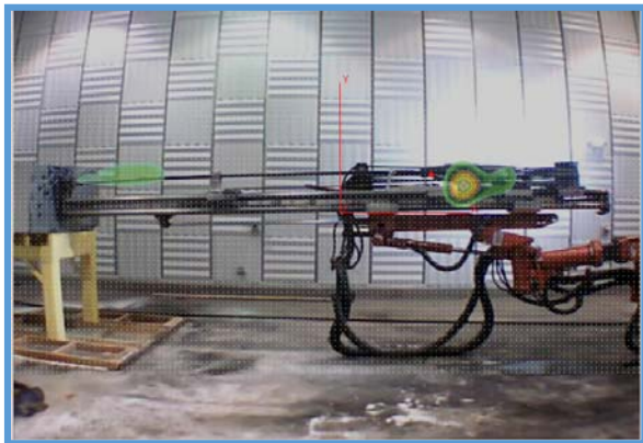
Figure 6 : Beamforming data collected just after the drill bit was fully collared, 2,500 Hz one-third octave band.
