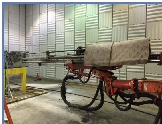
Figure 9 : View showing acoustic blankets draped over the drifter and hydraulic hose reel.
