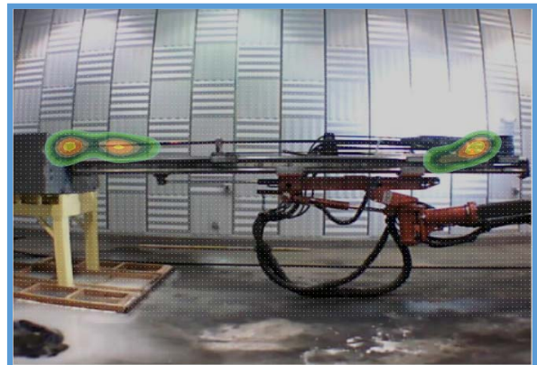
Figure 7 : Beamforming data collected near the end of the full hole depth, 2,500 Hz one-third octave band.
