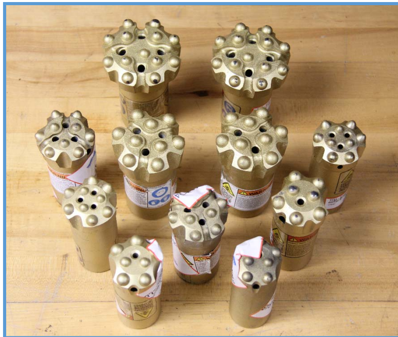
Figure 3 : Examples of the drill bits used during sound power testing
