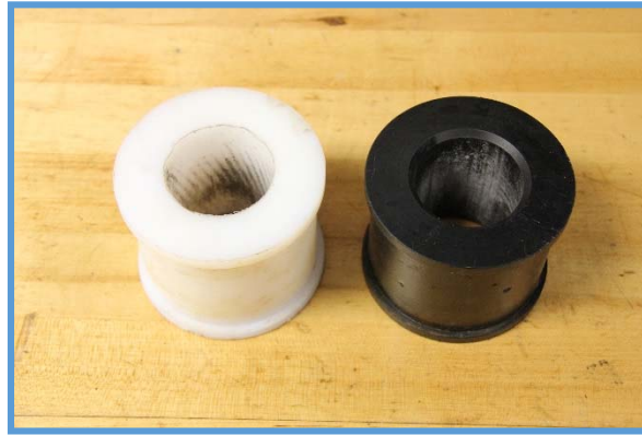
Figure 10 : Guide inserts used for proof of concept testing, made of UHMW-PE on the left (Insert #1), and Delrin ® on the right (Insert #2).
