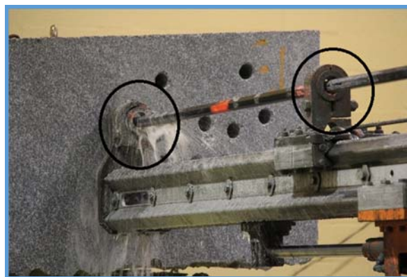
Figure 8 : Location of drill string guides.
