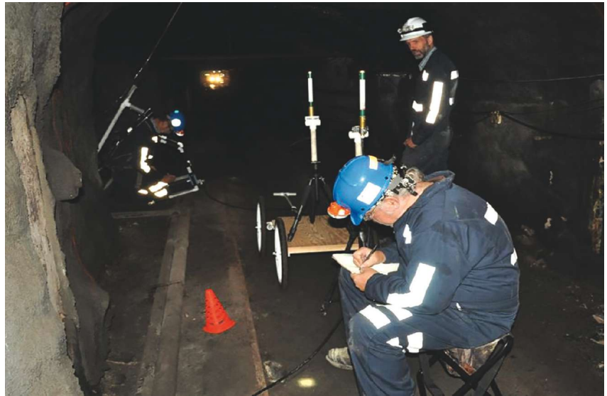
NIOSH researchers characterize signal propagation based on antenna orientation and location within a coal mine entry.
