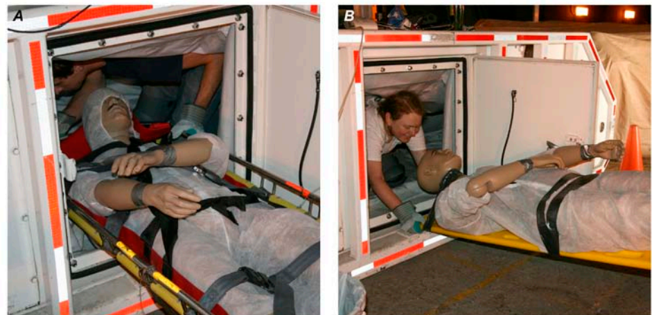
Figure 7: Moving the A) splint stretcher and B) full-length hard backboard stretcher into the inflatable RA airlock.
