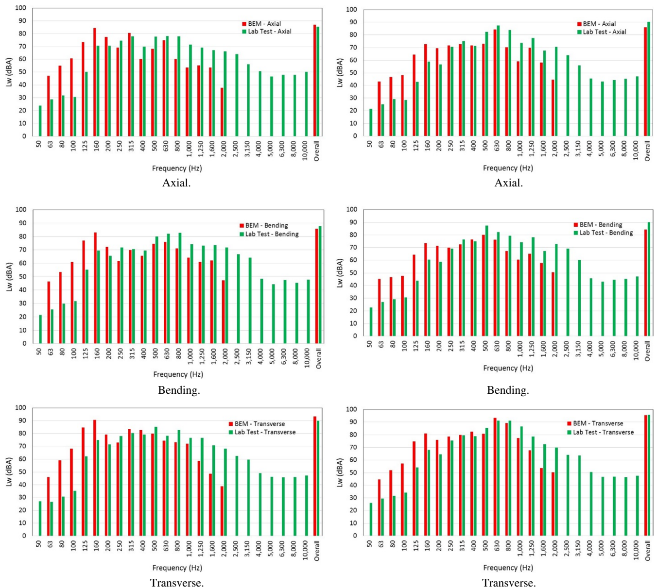
Fig. 15—Comparison of the sound power level computed from the BEM model and from laboratory measurements of a standard drum for Point 65.
