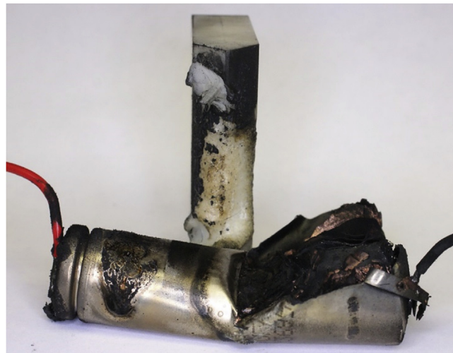
Fig. 6. Photograph of a ruptured CL cell that ignited the 20-L chamber atmosphere with a partially melted plastic wedge.
