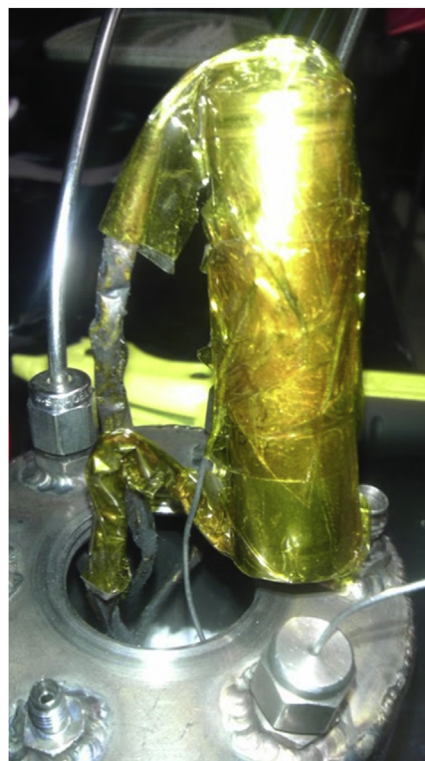
Fig. 5. Photograph of a kapton tape wrapped Li-ion cell prepared for placement within the AllCell ARC test chamber.
