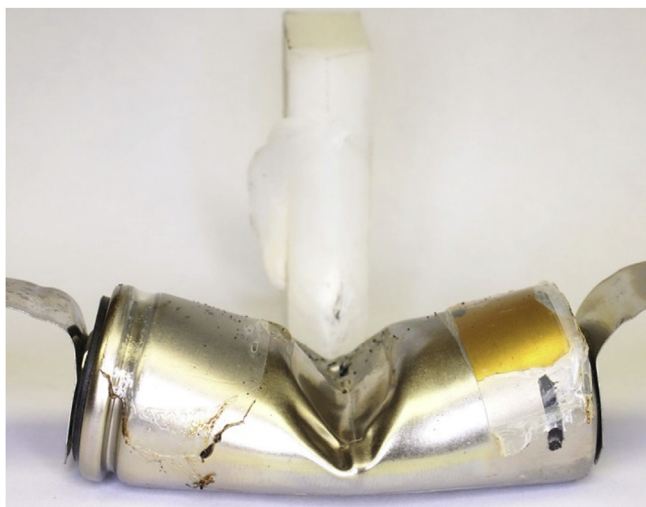
Fig. 8. Photograph of a crushed K2 cell that did not ignite the 20-L chamber atmosphere with a partially melted plastic wedge. The cell short-circuited internally.
