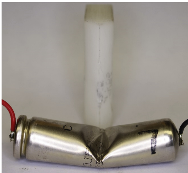
Fig. 7. Photograph of a crushed PDM cell that did not ignite the 20-L chamber atmosphere with a plastic wedge. The cell short-circuited internally.
