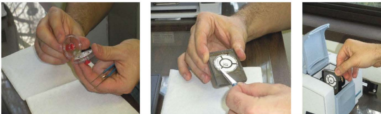
Figure 3 — Three steps for the new monitoring solution: (left) open the sampling cassette; (center) insert the cartridge in a holder; and (right) place the holder in the portable instrument.
