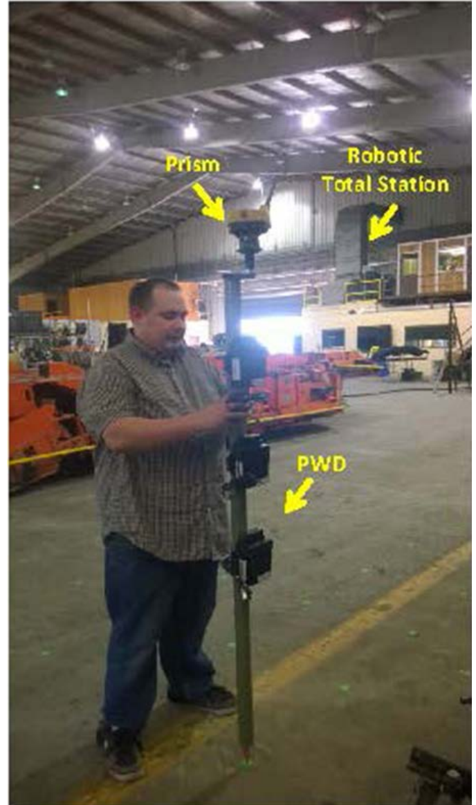
Figure 4. Personal wearable devices mounted on data collection pole.
