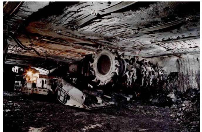
Figure 1. Continuous mining machine underground.
