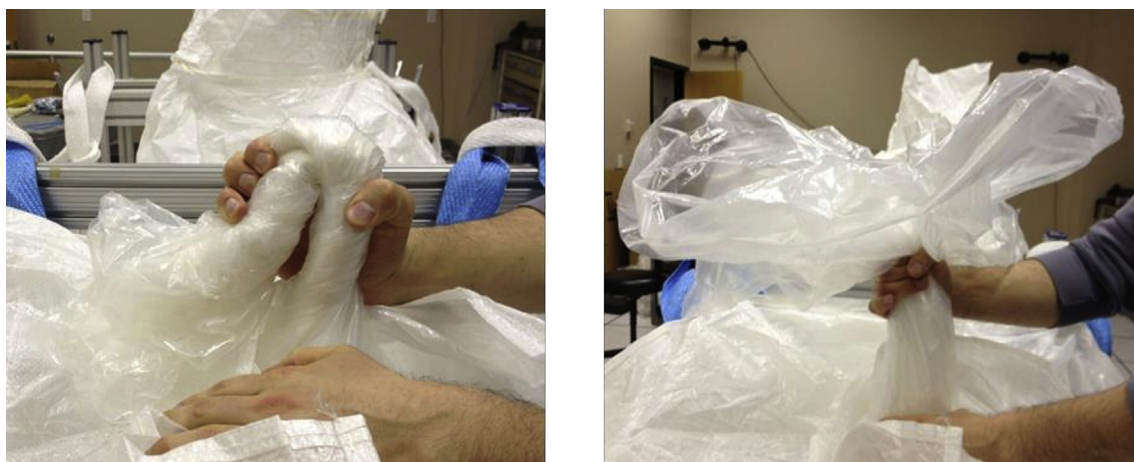
Fig. 2. Bag closing methods; snaking (left), flowering (right).
