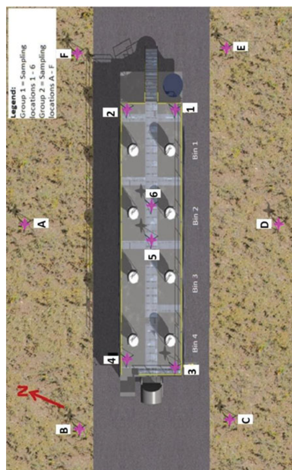
Figure 4. Air sampling locations for test of mini-baghouse. Computer rendering developed by Kenneth Strunk, NIOSH Spokane, and modified by Barbara Alexander, NIOSH DART.
