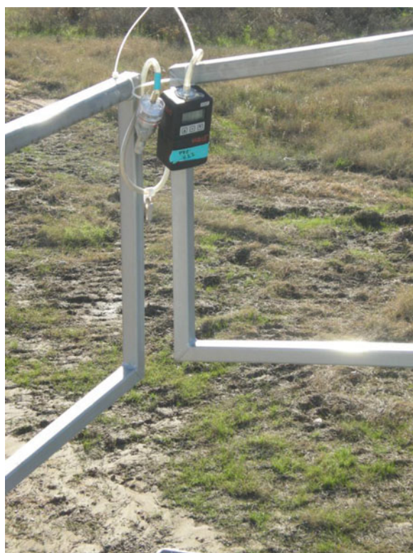
Figure 5. Air sampling train installed on upper corner of sand mover. Photo courtesy of Mike Gressel and Jerry Kratzer, NIOSH.
