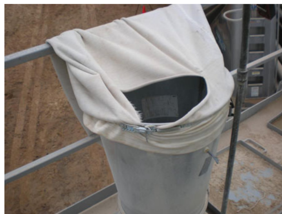
Figure 11. Failure of filter bag during test of mini-baghouse. Photo courtesy of Mike Gressel and Jerry Kratzer, NIOSH.
