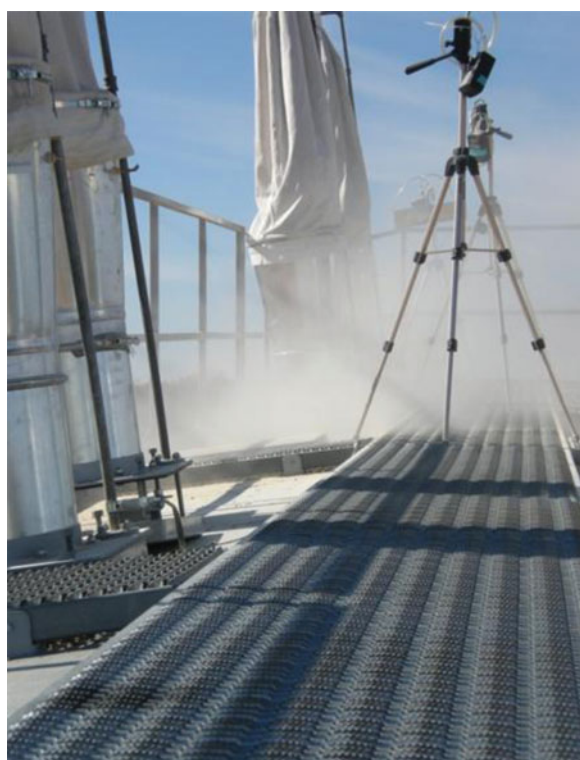
Figure 6. Sampling train located in the middle of the top of the sand mover during an uncontrolled trial run. Note visible cloud of silica-containing aerosols released from thief hatch opening when mini-baghouse is not in place. Photo courtesy of Mike Gressel and Jerry Kratzer, NIOSH.
