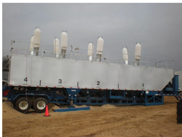
Figure 3. NIOSH mini-baghouse assemblies installed on eight thief hatches atop a sand mover during filling operations. Photo courtesy of Mike Gressel and Jerry Kratzer, NIOSH.
