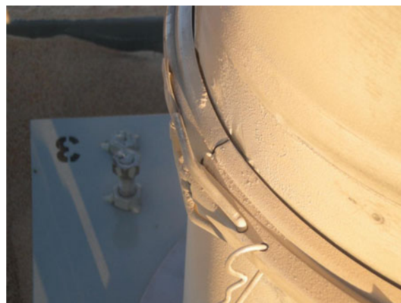
Figure 10. Dust leakage visible at the band clamp connecting two sections of ductwork on the mini-baghouse. Photo courtesy of Mike Gressel and Jerry Kratzer, NIOSH.
