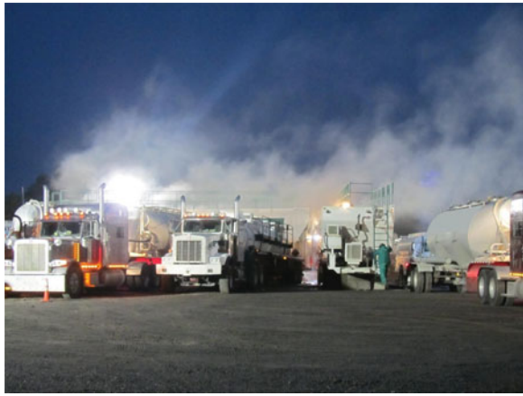
Figure 1. Clouds of dust are visible as sand trucks are unloaded at a hydraulic fracturing site. Photo courtesy of Michael Breitenstein, NIOSH.
