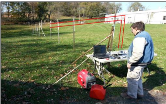
Fig. 5. Surface transmission line
