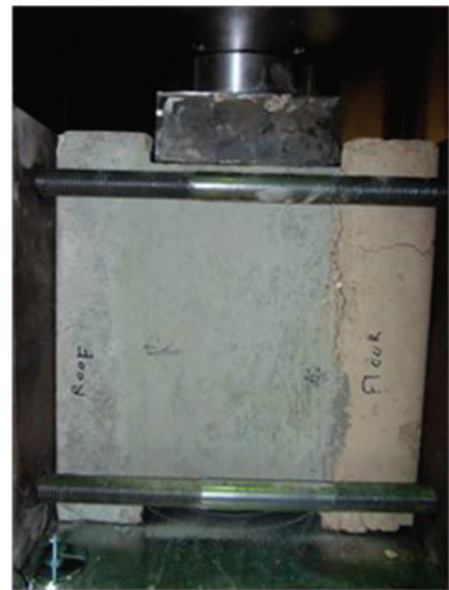
Figure 5 – Photograph of double direct shear test fixture for 0.084-m 2 (130-in. 2 ) test specimens in test machine showing cement foam material loaded by ram and concrete roof and floor blocks.
