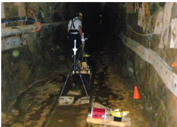
FIGURE 10. Conducting the propagation measurements in the hard-rock mine.
