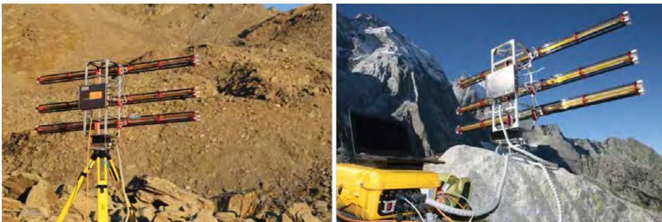
Figure 1. Examples of a portable radar interferometer mounted on a heavy-duty survey tripod (left) and on a simple 18 x 18 cm stainless steel plate (right).
