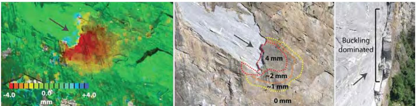
Figure 3. Detail of the radar interferometric deformation signal projected into a high resolution photogrammetric 3D model (left), contoured deformation field of the unstable rock block (center) and side-looking view of the unstable rock block showing a buckling mechanism (right)
