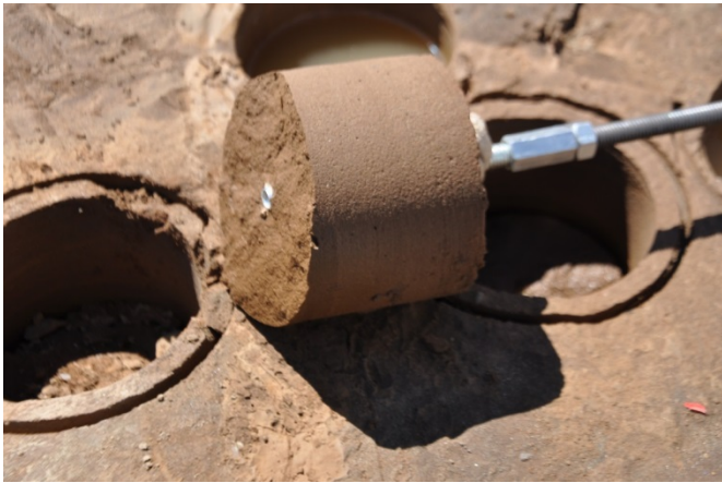
Fig. 21. Typical shallow tensile failure in the paste backfill.
