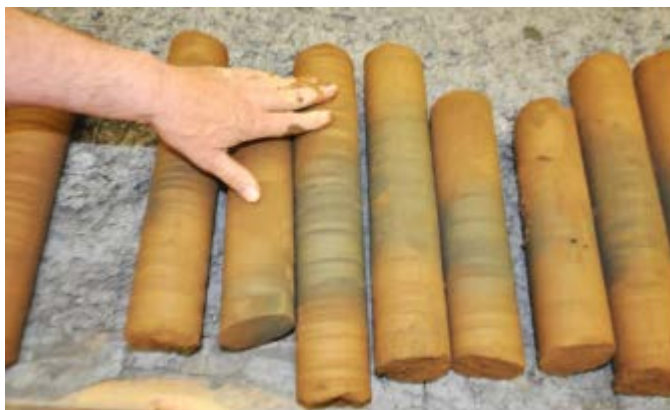
Fig. 4. Cores obtained from the small paste backfill slab.
