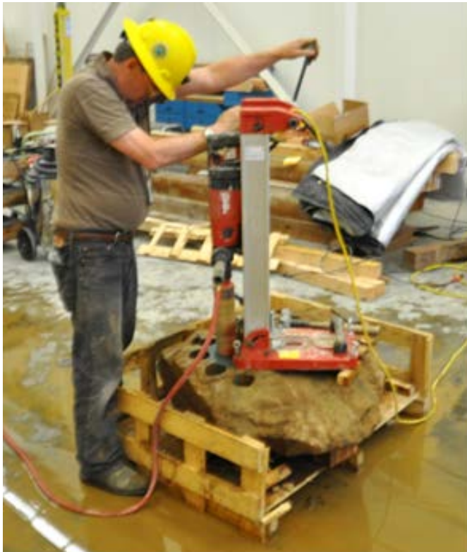
Fig. 3. Core drilling of the smaller paste backfill slab.
