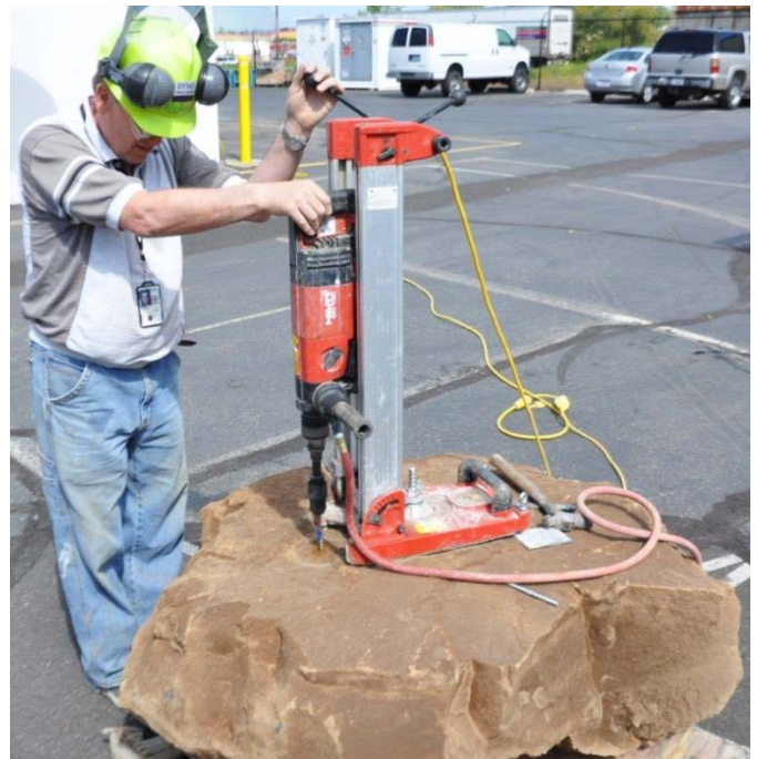
Fig. 11. Drill and stand attached to the backfill slab.
