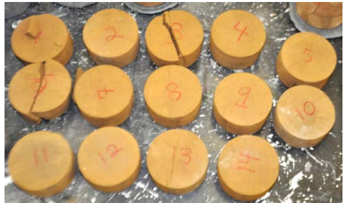
Fig. 5. Brazilian test specimens and typical failure.
