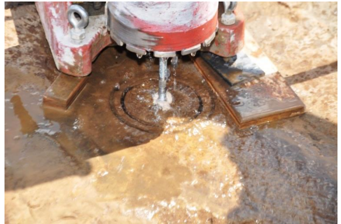
Fig. 16. Shallow kerf drilled around the test core using a 13cm (5 in) core bit.
