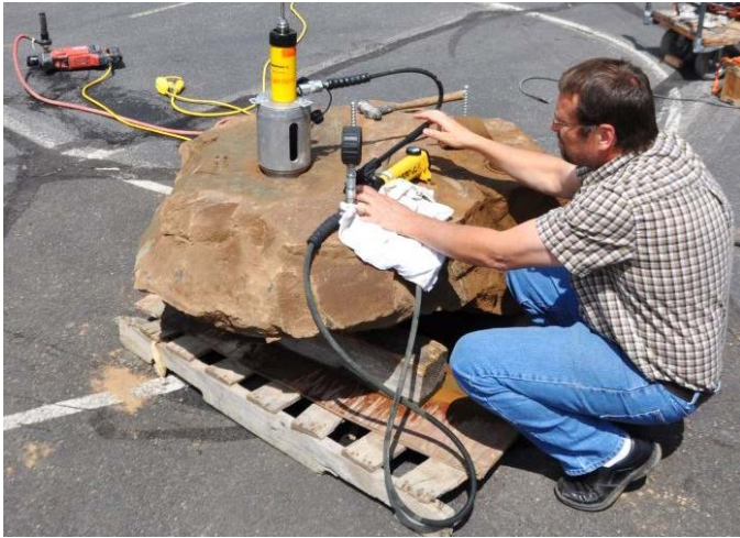
Fig. 20. Performing an in situ direct tensile strength test.
