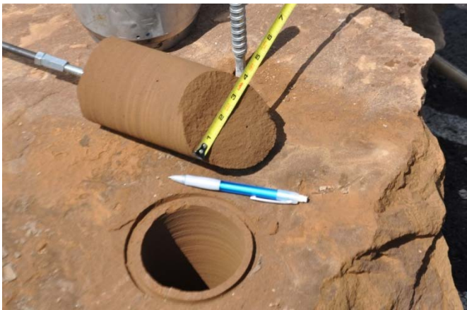
Fig. 22. Typical shear stress failure oriented about 45 degrees to the axis of the test core.
