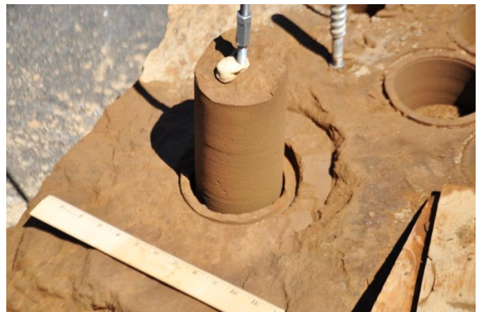
Fig. 25. Removing the longest test core from the backfill slab.
