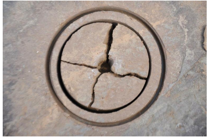
Fig. 24. Typical failure when the epoxy anchored bolt is pulled out of the slab.
