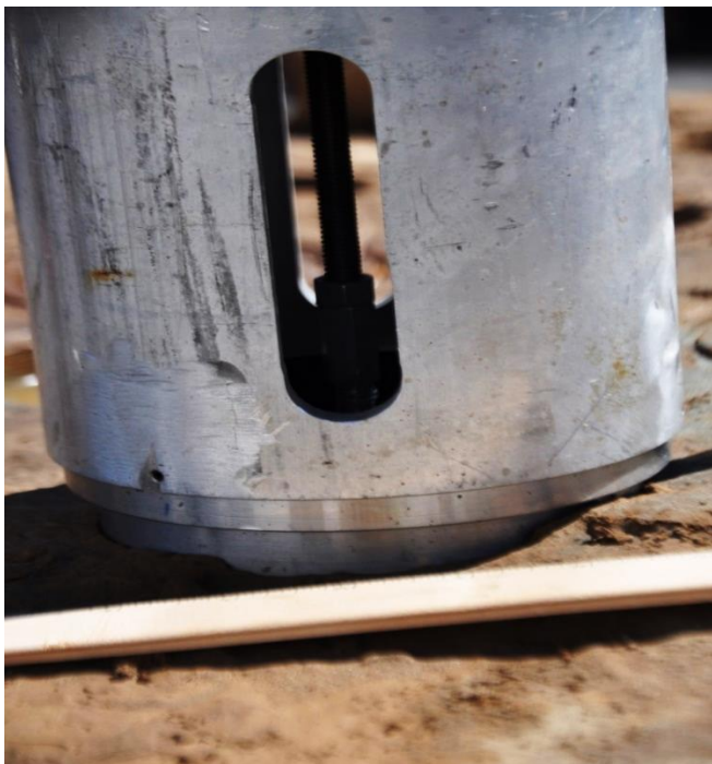
Fig. 18. Seating ring of pulling fixture inserted into kerf.
