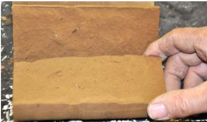
Fig. 7. Typical splitting tensile test failure.
