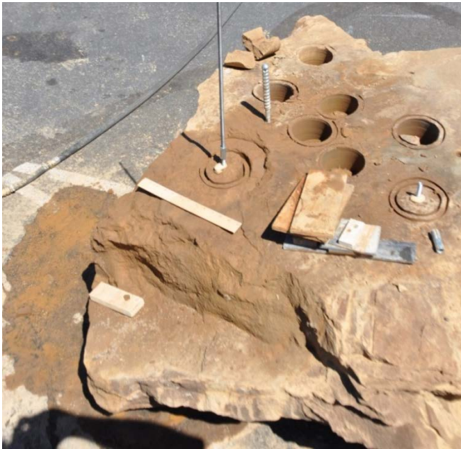
Fig. 27. Paste backfill slab near the completion of in situ direct tensile testing.
