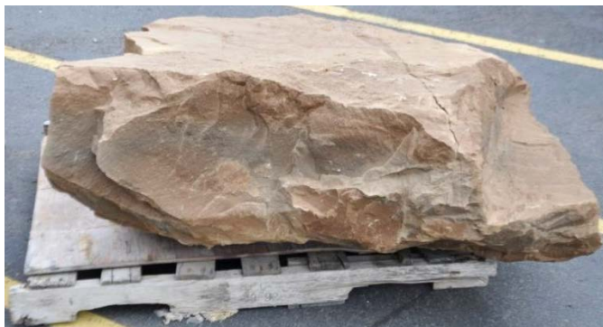
Fig. 10. Larger paste backfill slab on a wood pallet.
