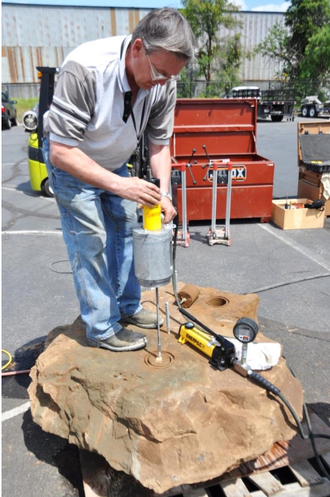
Fig. 17. Hydraulic ram and pulling fixture being inserted over the all-thread.
