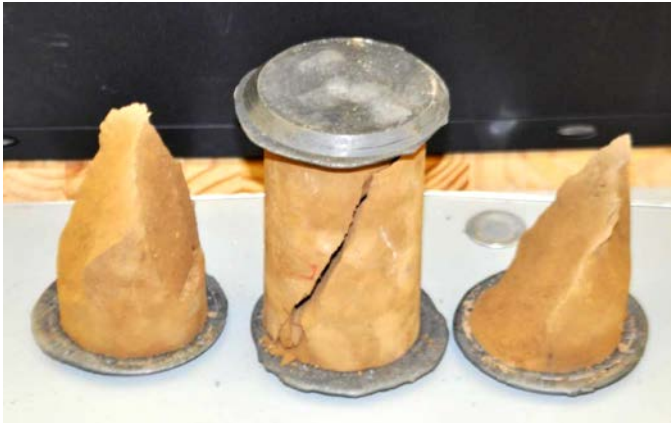
Fig. 28. Typical failure for unconfined compression tests.
