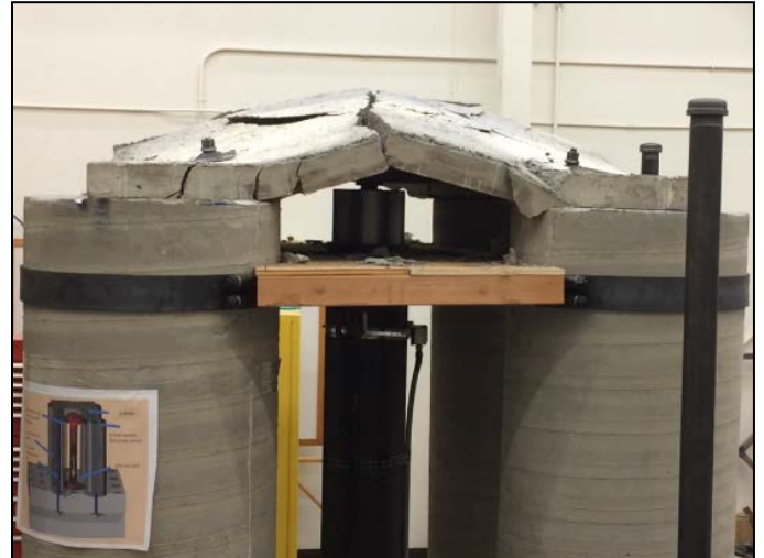
Figure 9. HEHD panel test sample loaded to 10-in displacement (side view).
