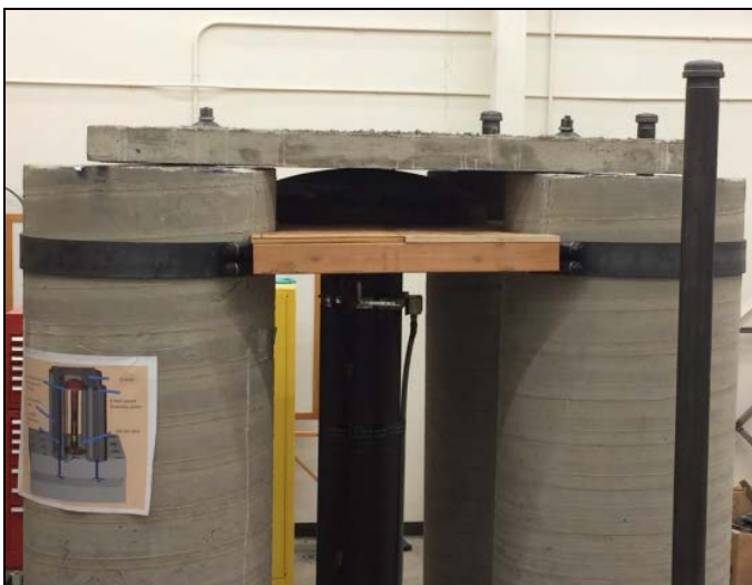
Figure 8. HEHD panel with loading head in position for test to start.
