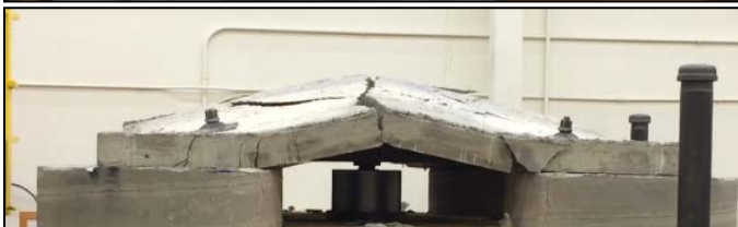
Figure 12. HEHD panel test sample initial loading to 6 to 8-in displacement (oblique and side view).
