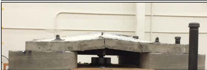
Figure 11. HEHD panel test sample initial loading to 2 to 6-in displacement (oblique and side view).
