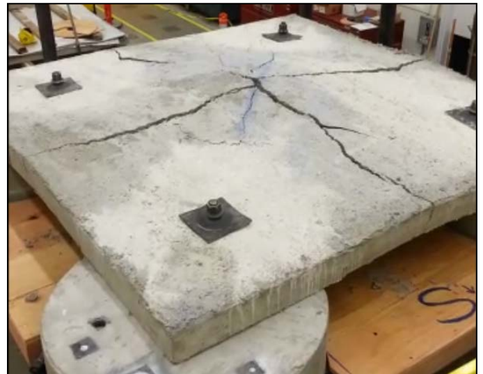
Figure 10. HEHD panel test sample initial loading to 0 to 2-in displacement (oblique and side view).
