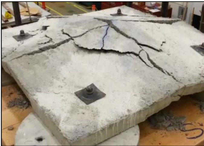
Figure 11. HEHD panel test sample initial loading to 2 to 6-in displacement (oblique and side view).
