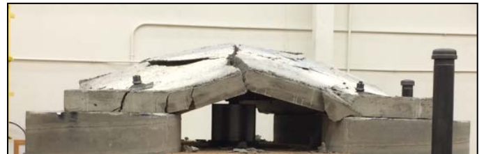
Figure 13. HEHD panel test sample initial loading to 8 to 10-in displacement (oblique, plan and side view).
