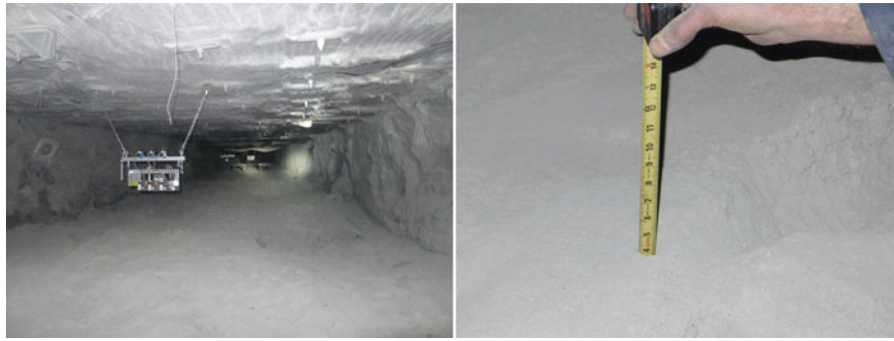
Figure 2. Rock dust deposits on the roof, ribs, and mine floor at a field sampling location in a continuous miner air ventilation return.
