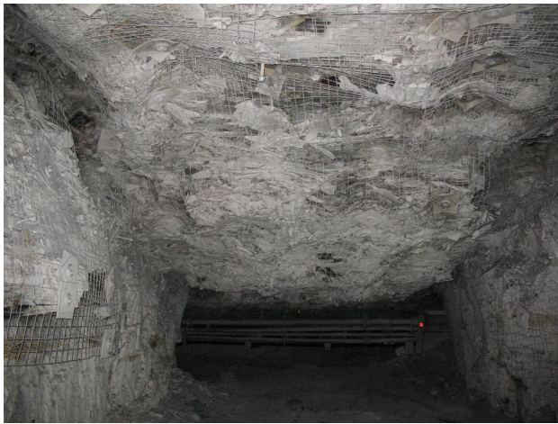
Fig. 13 Example of roof screen used to control deteriorated roof
