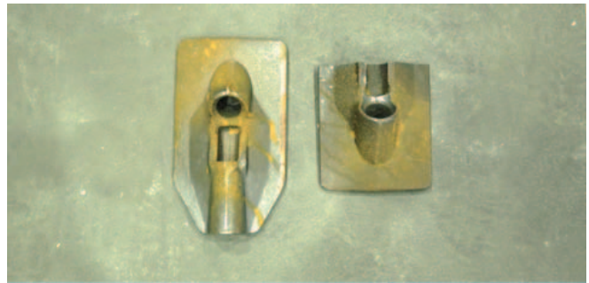
Figure 2. A bar shoe and a shoe cut for the top of the fixture.
