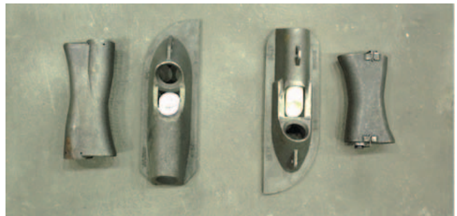
Figure 3. Shoes and dog bones for 0.7-inch cable (l) and 0.6-inch cable (r).
