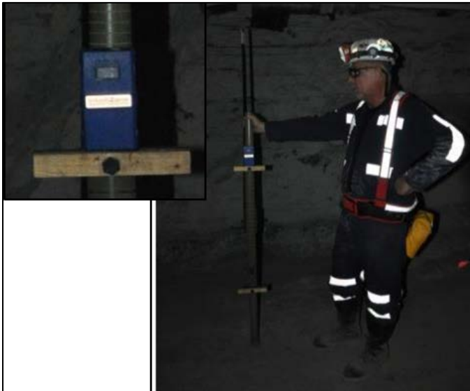
Figure 3. Researcher holding the reference pole while conducting a test (Inset: PWD attached to reference pole).
