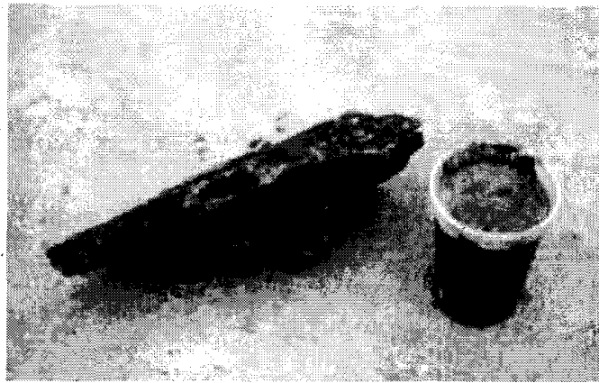
Figure 3 – The effect of water on a moisture-sensitive shale (from Mark and Molinda 2007).
