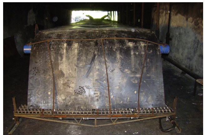
Fig. 2 – Setup of conveyor belt and ignition gas burners.
