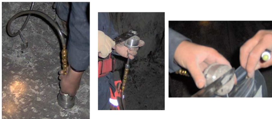
Fig. 8. Pump sampler used to obtain dust samples 2.5-mm, 1.6-mm, and 0.8-mm deep.
