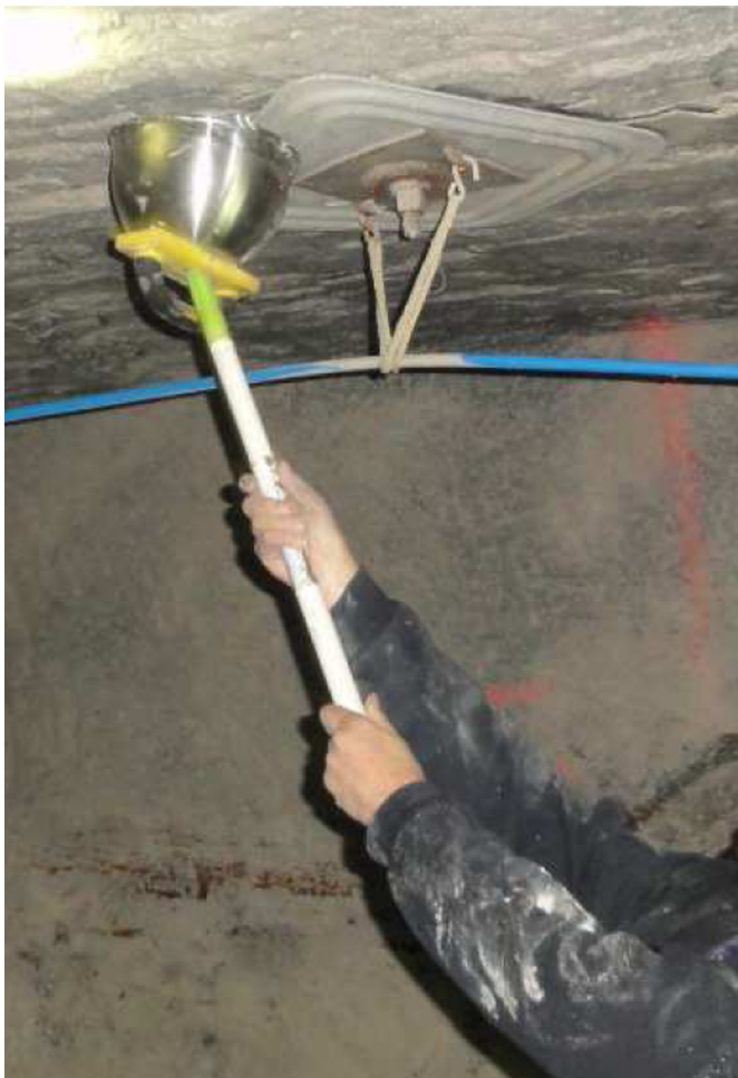
Fig. 2. Collecting a roof sample using the bowl and brush with a handle.
