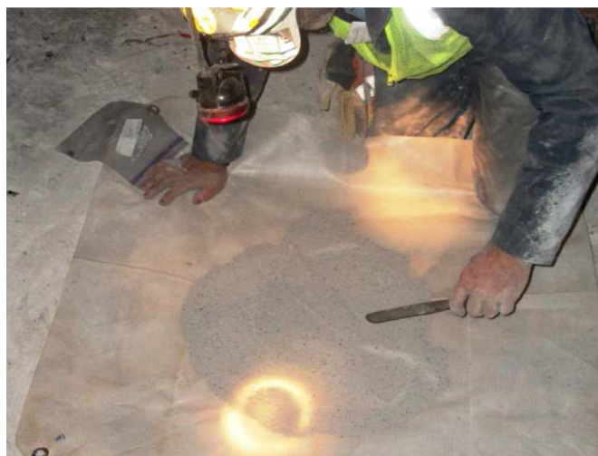
Fig. 6. Coning and quartering of the collected floor dust.
