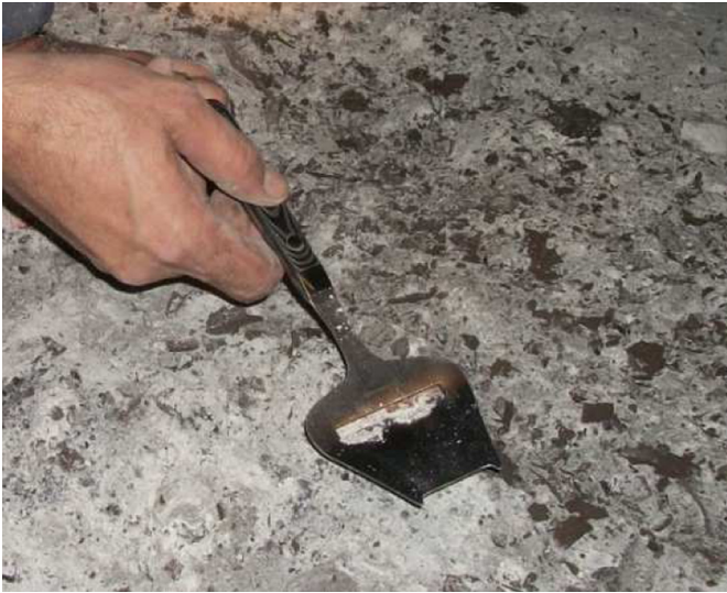
Fig. 7. A cheese planer is used to collect a 3-mm depth dust sample from the floor.
