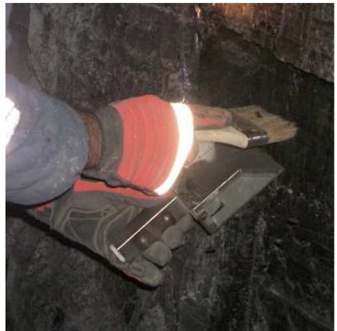
Fig. 3. Brush and pan used for sample collection on ribs.
