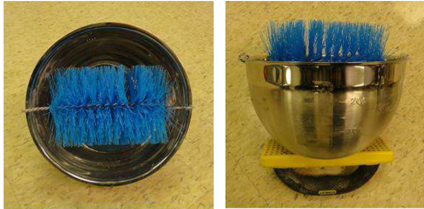
Fig. 1. Bowl and brush configuration mounted on a mop head to collect roof samples.
