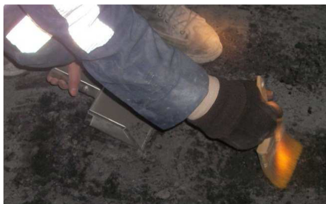
Fig. 5. A brush and pan were used to collect dust from the floor up to 2.5 cm deep.
