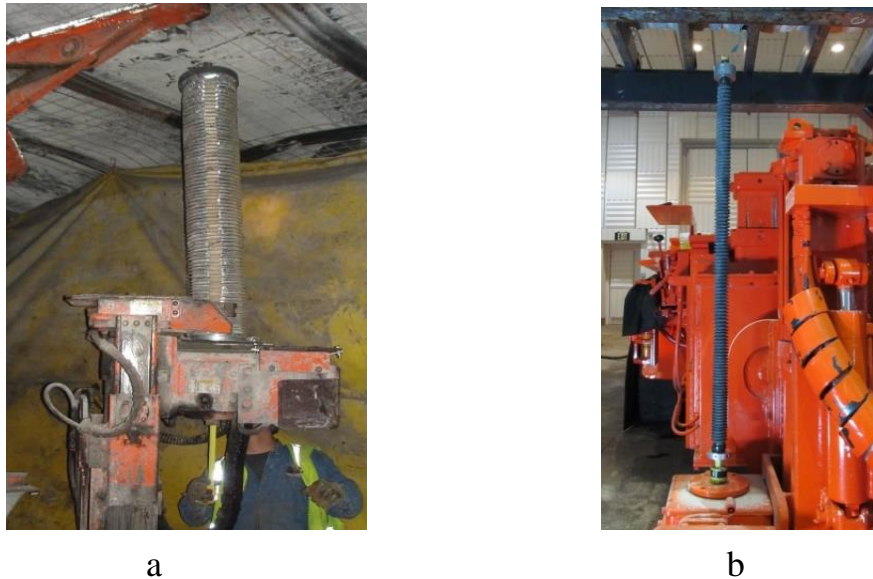
Figure 1: a) Prototype CDSE installed on a roof bolting machine in an underground coal mine. b) Redesigned CDSE installed on a roof bolting machine in the NIOSH OMSHR hemi-anechoic chamber.
