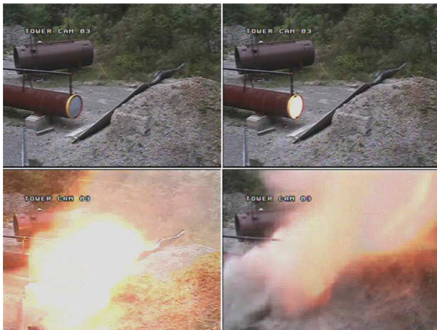
Figure 4 Video recording of GETF test explosion sequence with frames about 1/30 second apart. These show the tube with plastic, the diaphragm prior to rupture, the arrival of the detonation wave, and venting of burning gases.
