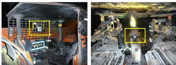
Figure 2. Dust sampling packages located on a shuttle car (left) and on a roof bolter (right).
