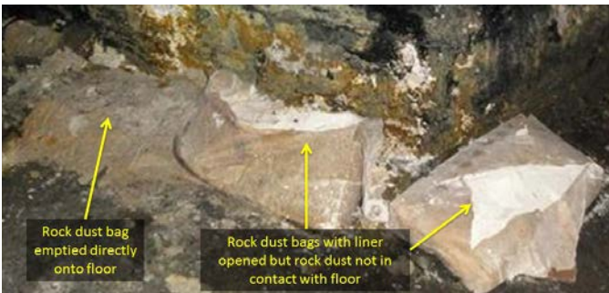
Figure 2. Three bags of rock dust placed at one location in the SRCM.
