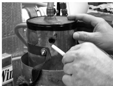
Fig. 2 Apparatus used to introduce cigarette smoke into chamber.
