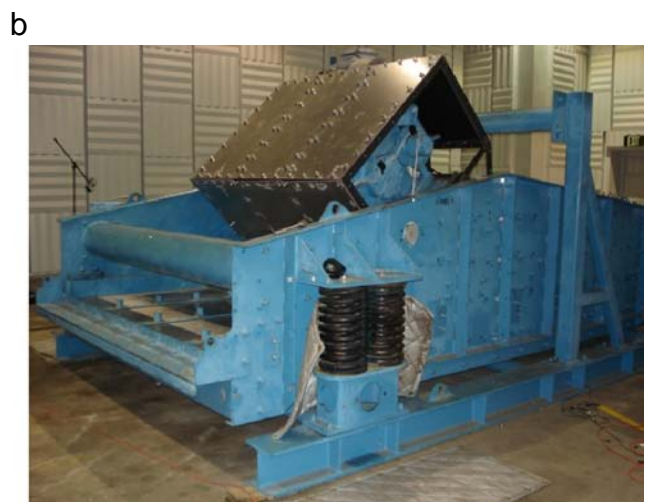
Fig. 9—Steel frame for the second enclosure showing (a) one frame section and (b) the entire frame assembly with most panels installed on a vibrating screen.
