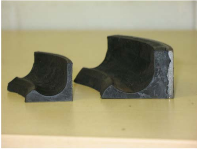
Fig. 4—Examples of small (left) and large (right) spring inserts. Note that the metal backing plate has been removed from the small spring insert.
