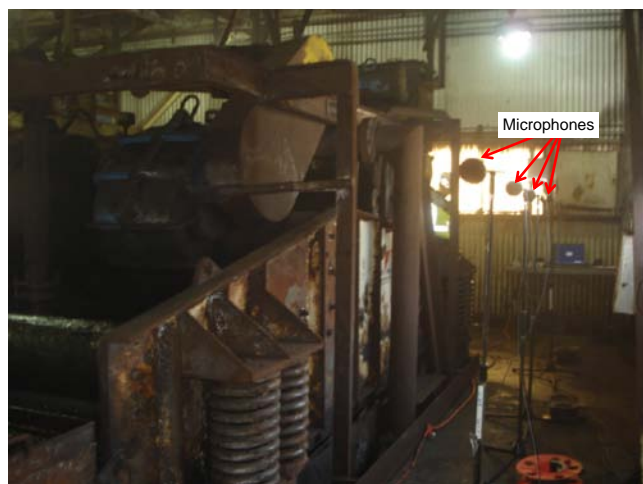
Fig. 17—Microphone positions 3–6 on the left side of the screen.
