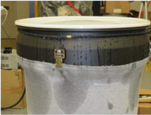
Fig. 2 Simulated miner (barrel) with porous hose delivering water droplets
