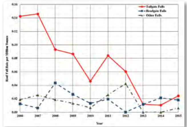
Fig. 1 Roof-fall rates that resulted in a gateroad blockage or other nearby fall.
