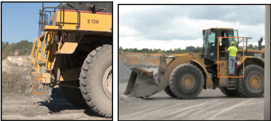
Fig. 2. Fall from equipment. The left image displays a slip, trip, and fall (STF) hazard without a person, where the bottom rung of the ladder on the haul truck is missing. The right image displays a STF hazard with a person, where the mineworker cannot maintain three points of contact while climbing the ladder because he is carrying a lunchbox. Both hazards were included in the laboratory study only.
