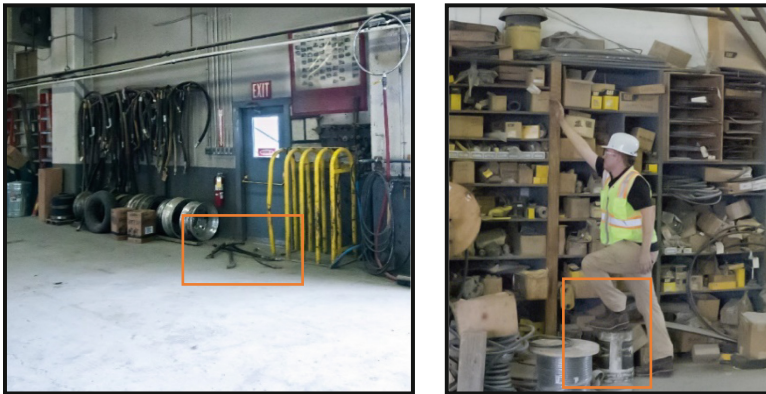
Fig. 1. Fall to walk way or working surface. The left image displays a slip, trip, and fall (STF) hazard without a person, where the pipes and cables inside the orange rectangle are the hazard. The right image displays a STF hazard with a person, where a bucket being used as a step is the hazard. Both hazards were included in the laboratory and training data collections.
