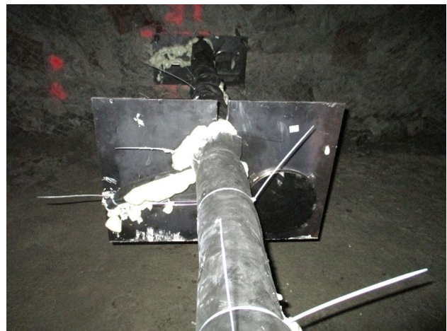
Fig. 14 Contact pressure cell (manufactured by Geokon, Inc.) mounted on a closure meter anchor plate
