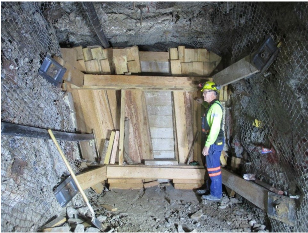
Fig. 5 Photograph in the 6350 level (1935 m below shaft collar), 12-stope east showing fill fence and 0.3-m gap between consecutive backfilled levels
