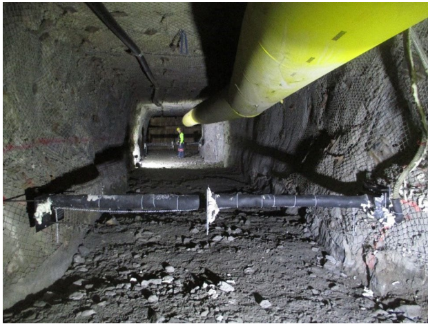
Fig. 13 Typical backfill instrumentation setup used to monitor stope wall convergence and horizontal fill pressure
