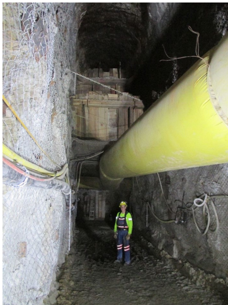
Fig. 6 Photograph in 6350 level (1935 m below shaft collar), 32 slot showing current cut and remaining fill fences from the two backfilled cuts above
