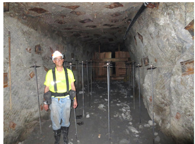
Fig. 4 Preparing the 5550 level (1690 m below shaft collar), 11-stope east for backfilling
