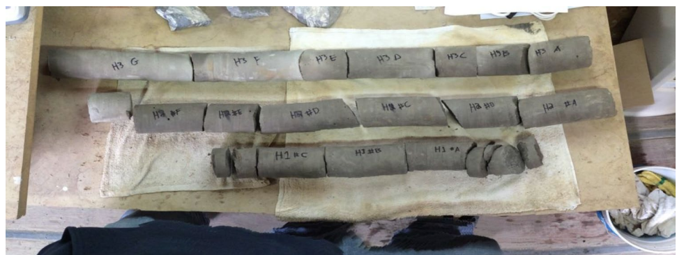
Fig. 11 Breaks observed in backfill core are primarily due to drilling-related effects with the exception of the fractures at the collar
