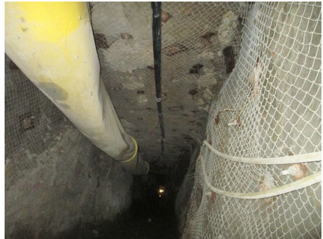
Fig. 7 Photograph in 6350 level (1935 m below shaft collar), 12-stope east showing reinforced CPB back
