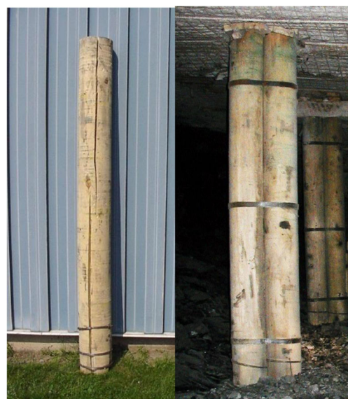
Fig. 6 Example of yielding post (left) and cluster of three yielding posts (right)
