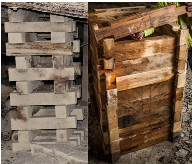
Fig. 4 Example of a four-point crib (left) and an engineered wood crib (right)
