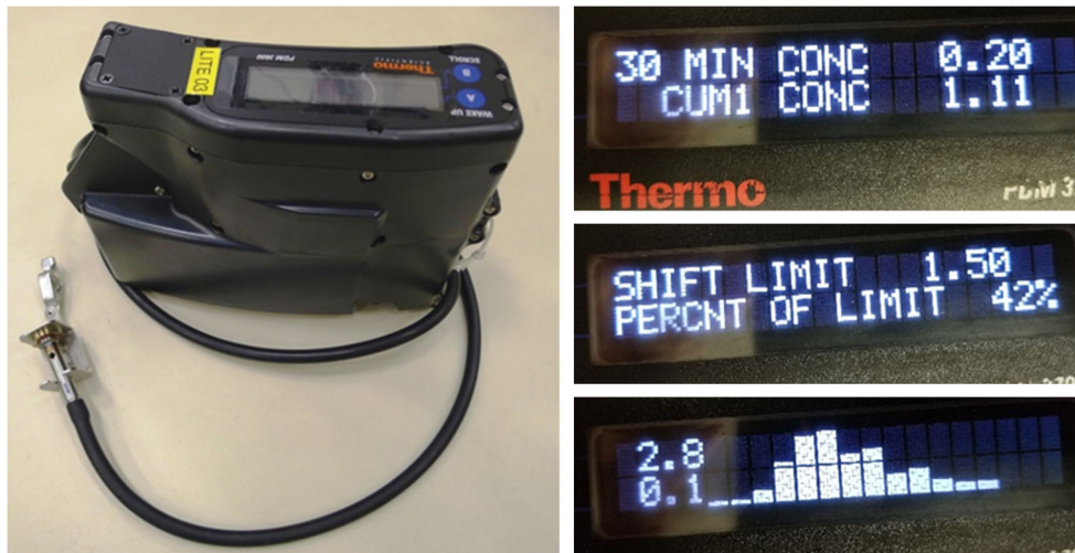
Fig. 4 PDM 3700 dust monitor (left) and information screens available (right). The screen view shown in the top right photo in Fig. 4 provides the average respirable dust concentration for the previous 30 min of sampling, in addition to the average cumulative concentration from the beginning of the sampling shift. The screen shown in the middle right
