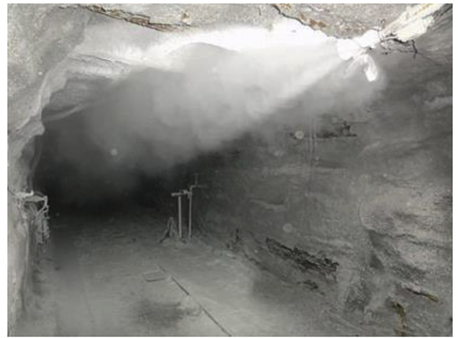
Fig. 2. Air-dust discharge through a 2-in (5.1-cm) diameter tube attached to the roof 7.25 ft (2.2 m) above the floor.
