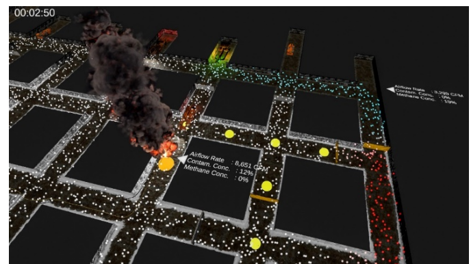
Figure 6. An overhead depiction of a section of a mine with methane liberation coming from the face of the second entry and a fire two crosscuts outby as modeled by MFIRE. The small particle system represents the airflow velocity and methane concentration (i.e. blue = inert, red = explosive, white = none). The large spheres indicate level of contaminant by size and color (i.e. bigger = higher concentration; red = high, white = none).
