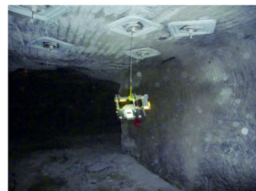
Fig. 2. A typical sampling package consisting of a pDR-1000 and two gravimetric samplers used by NIOSH.
