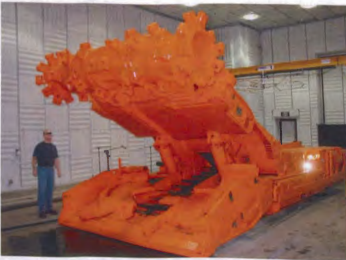
Fig. 12.20 CMM in the NIOSH hemi-anechoic chamber with overhead microphone array.
