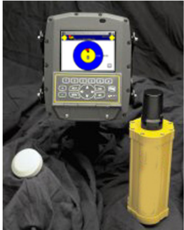
Figure 2. GPS system components. Left to right: GPS antenna, computer and display with integrated receiver, and IP radio.
