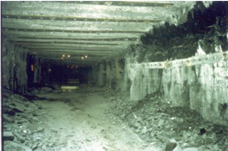
Figure 10.11 Tailgate abutment zone outby the face support with cable bolts (note the pillars are already sloughing on both the pillar (right) and coal panel (left)).
