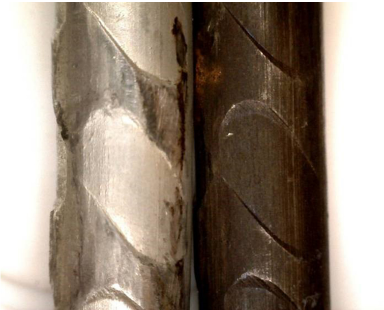
Figure 10.19 Indented galvanized PC-strand (left) and bright indented PC-strand (right).
