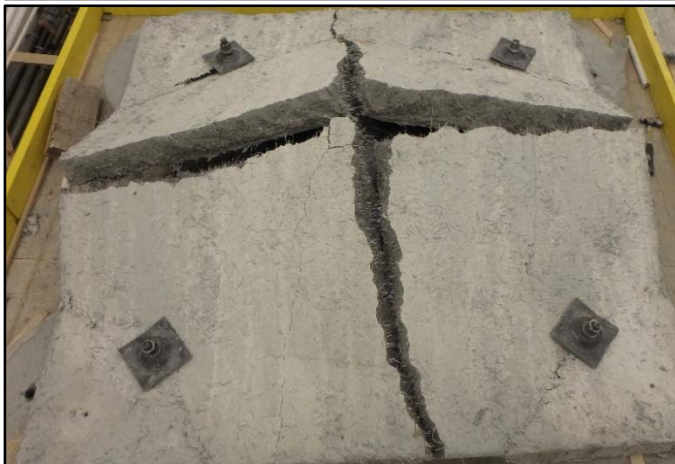
Figure 18 Post-test photos of a post-bolted, fiber-reinforced (11.7-lb/yd 3 ) shotcrete panel showing (top) shotcrete providing stable platform for bolt head to resist movement, and (bottom) predictable fracturing between bolts, identical to post-bolted, mesh-reinforced panels.
