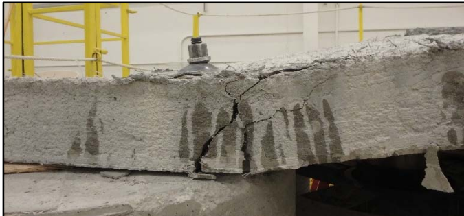
Figure 17. Post-test photo of a post-bolted, fiber-reinforced (5-lb/yd 3 ) shotcrete panel, showing fracture pattern similar to unreinforced shotcrete.
