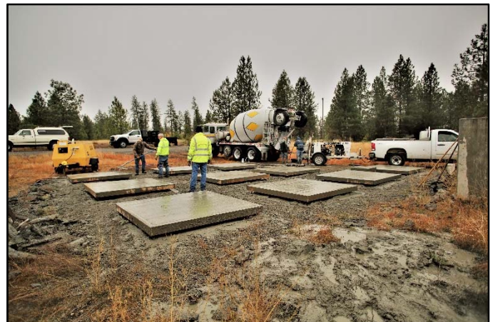
Figure 11. After shotcreting, the panels were screeded and floated to a uniform thickness to provide consistent test results.
