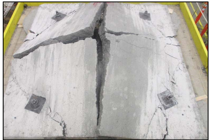
Figure 15. Post-test photo of a panel constructed to represent post-bolting of mesh-reinforced shotcrete showing complete tensile failure of wires spanning the shotcrete cracks.
