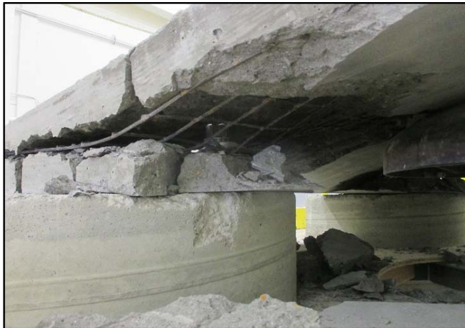
Figure 14. Post-test photo of a panel constructed to represent spraying a flash coat of shotcrete, installing mesh and bolts, and additional shotcrete showing separation of shotcrete at mesh interface.
