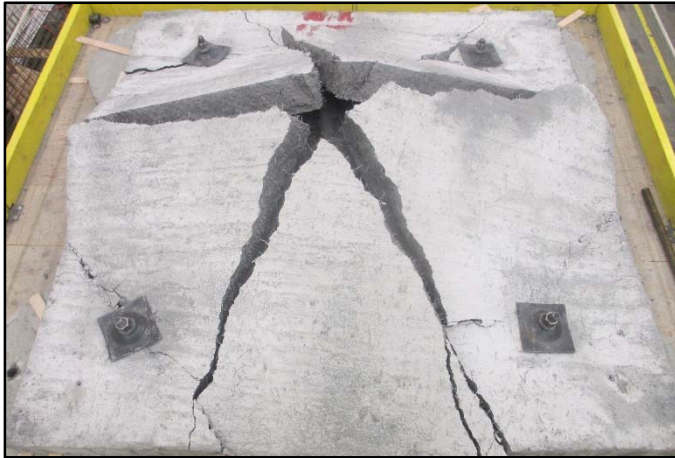
Figure 17. Post-test photo of a post-bolted, fiber-reinforced (5-lb/yd 3 ) shotcrete panel, showing fracture pattern similar to unreinforced shotcrete.
