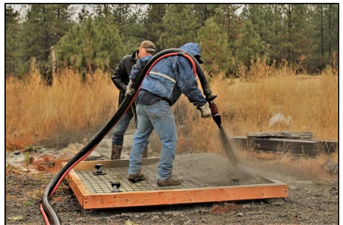
Figure 10. Shotcrete being applied by a certified nozzle operator over mesh and bolts plates. Plastic spacers were used to maintain access for bolting to the test frame after curing.
