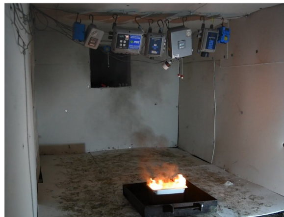
Fig. 2. Diesel fuel fire test setup.
