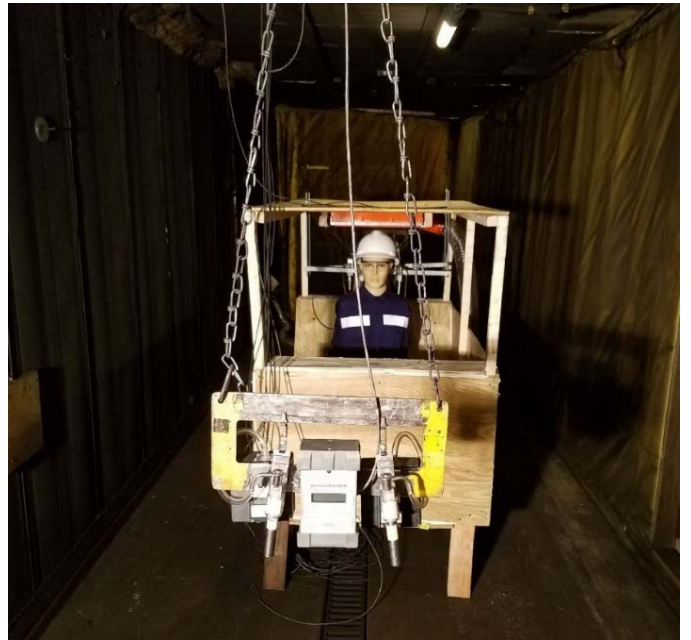
Figure 4. Photo showing the setup of the center-drive cab for testing with the manikin used for centering the CAC over the shuttle car operator.
