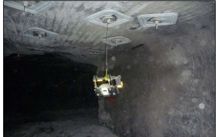
Figure 2. A typical sampling package consisting of a pDR-1000 and two gravimetric samplers used by NIOSH. The pDR-1000 is in the middle of the rack with the gravimetric samplers located adjacently on each side of the pDR-1000.
