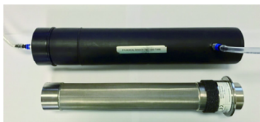
Fig. 6. Cylindrical tube and fiber optic sensor.
