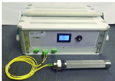
Fig. 1. RSL fiber optic methane detection system.
