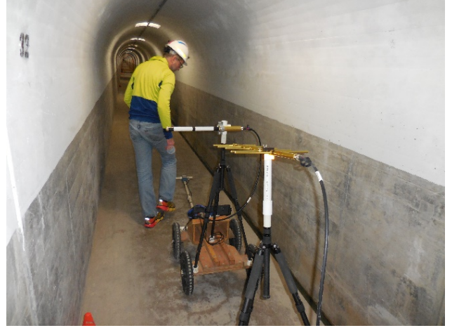
Figure 1 – Measuring the influence of antenna pattern in concrete tunnel
